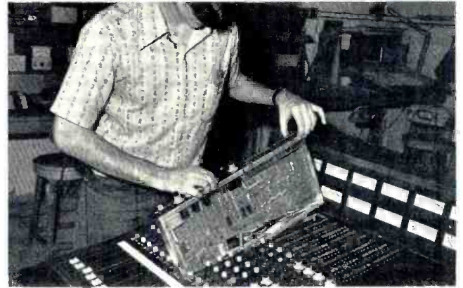
Gately consoles are constructed with standardized modular design. Each module can be slipped in and out as shown. Also seen is the module's single board. A master mother board is in the console.
