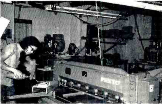
Here's an overall view of the sheet metal shop. All sheet metal work is done in-house including plating and etching of panels and components.
