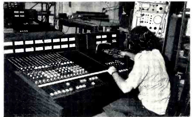
In these two photographs the console construction area is shown. Gately makes even the cabinets in his woodworking shop. With modules and components inserted, each console is given a painstaking shakedown before it goes out the door. We were told that it takes an average of seven men working one month to create a finished console.
